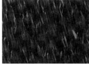
Figure 1: The structure of our AFLC cell which comprises of two sets of domains oriented at an angle of approximately 17^\circ relative to each other.
